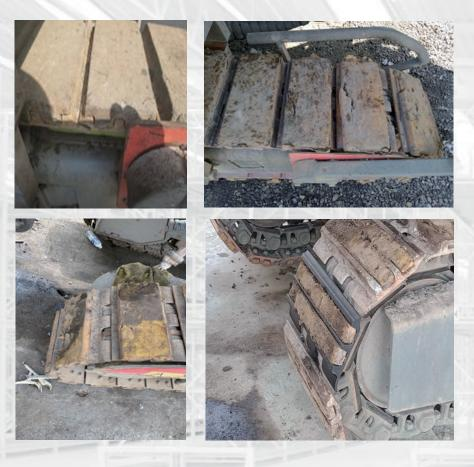
③ Chinese customers use Chinese brand polyurethane pads, which are too hard and have no stiffness. The pads cracked and fell off in about 3 months:
